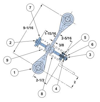
The #26W-3 One-piece Pan Arm Assembly replaces the #25W-3 three-piece assembly. Items 8 and 9, coil springs, are used for amplification of stroke only. Booster springs are used with applications to hold up the pan under heavy loads.
